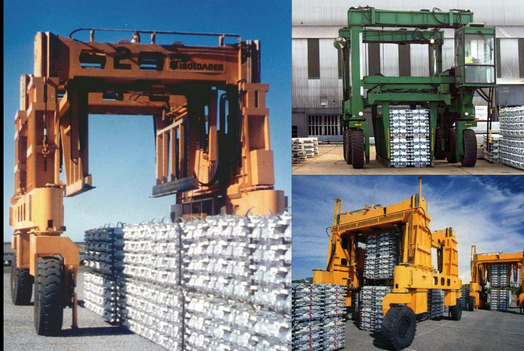
Spreaders with grab arms that squeeze in from the side can handle multiple ingot bundles without the need for additional strapping.
