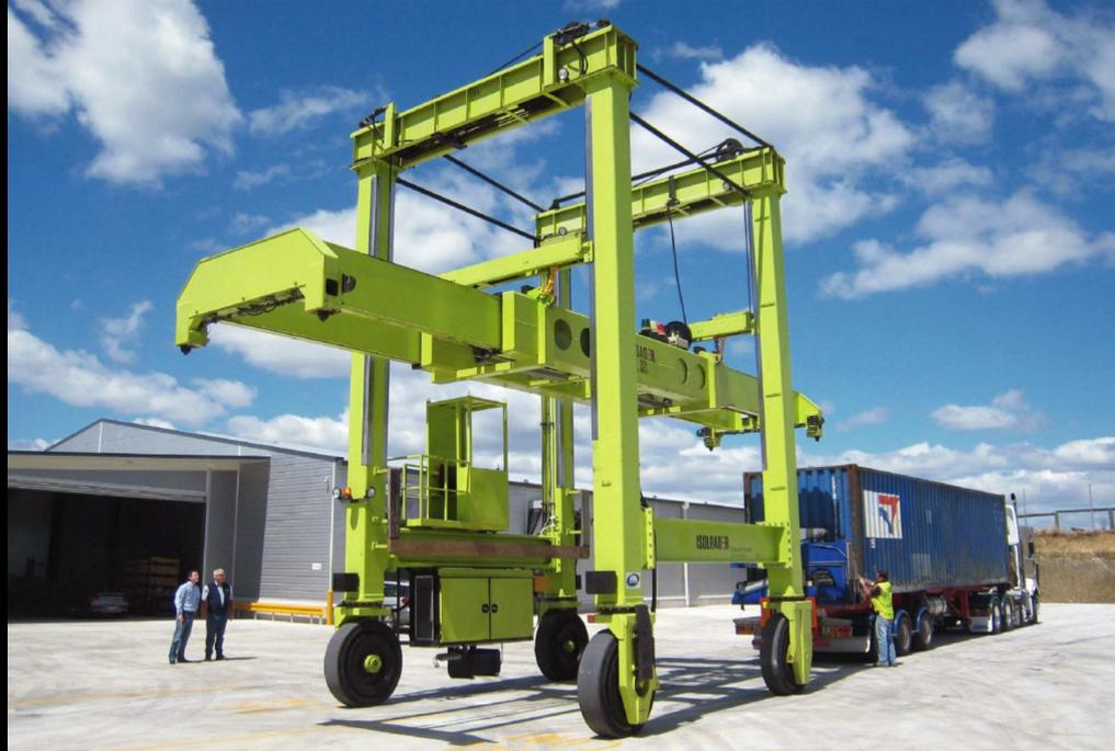
An economical mini straddle with proven dependability. Designed for warehouses, factories, distribution centres and trucking terminals requiring a single machine with flexible capabilities and minimal requirements. Comes in 1-high and 2-high models.
