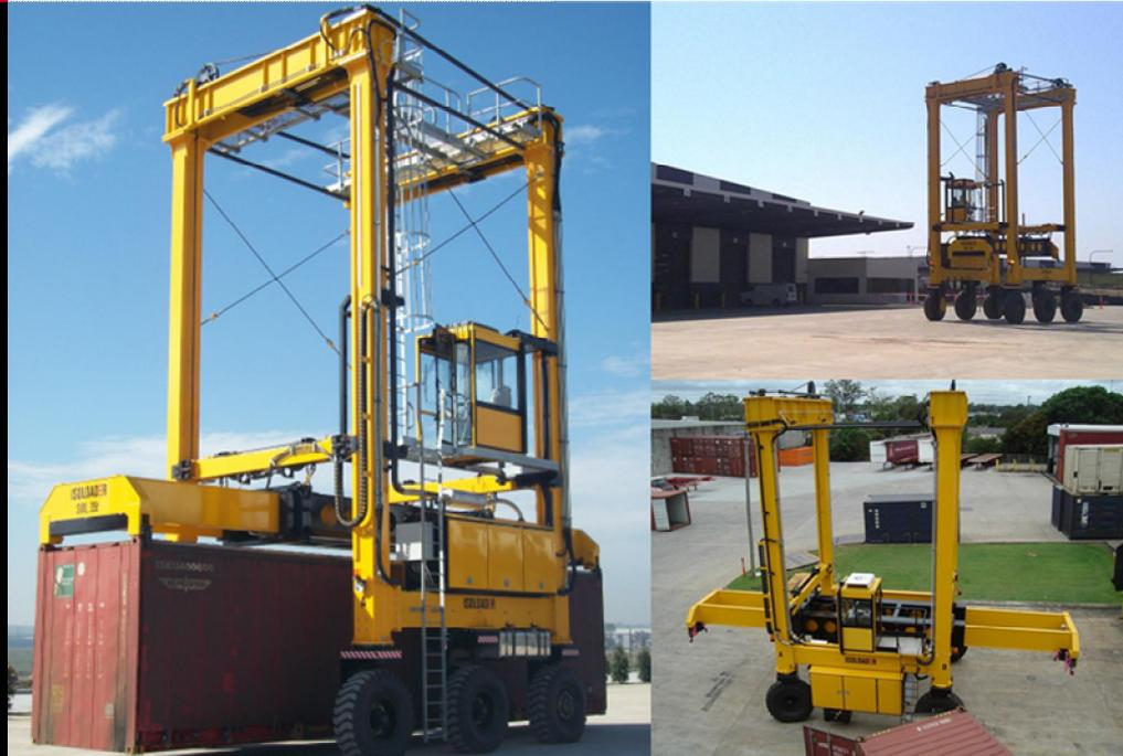
Isoloader's 3-high Transporter is 2/3rds the weight of a forklift, with half the fuel consumption and a fraction of the pavement costs.
